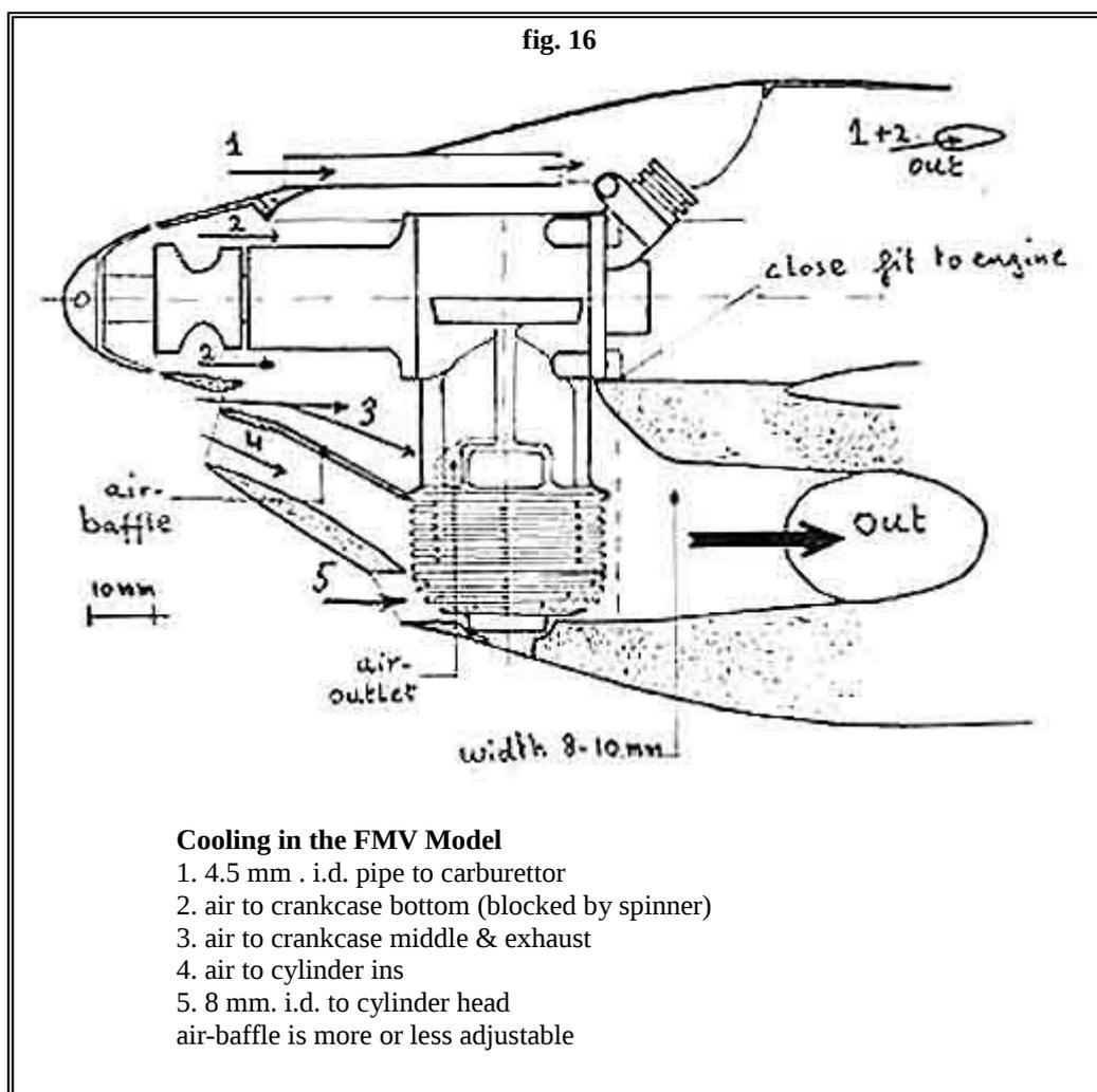
The 4.5 mm i.d. "pipe" directing to the carburetor is extremely important in our view. Air from a constant temperature is the only way to get constant needle settings. The only air of constant temperature is air directly from outside and this is also the coolest air we can get.
