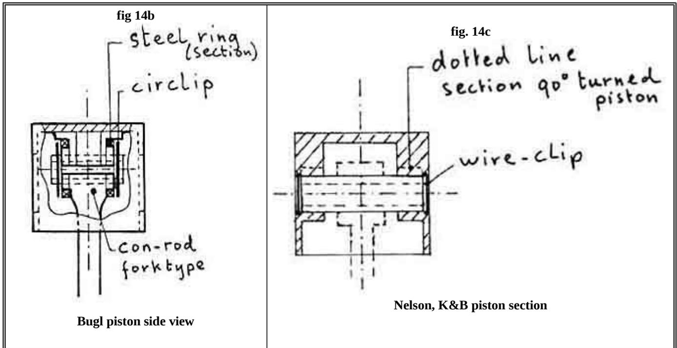
The piston pin in the FMV is kept in place by a wire clip of 0.6 mm diameter going through the pin into the piston, see fig. 14a. The thing looks nice and simple, but needs further improvement in order to enable the separation of the con-rod and the piston in the motor. With our small end construction it is quite a hard job to get the con-rod of the shaft with the piston on.
