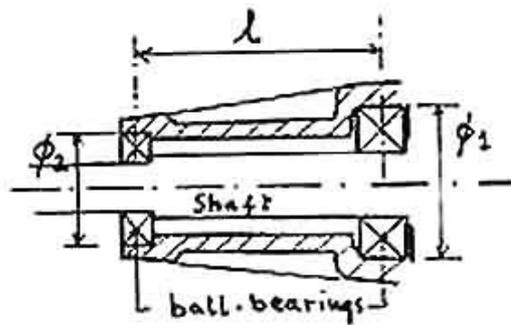
Shaft and bearings in an aluminium crankcase.
