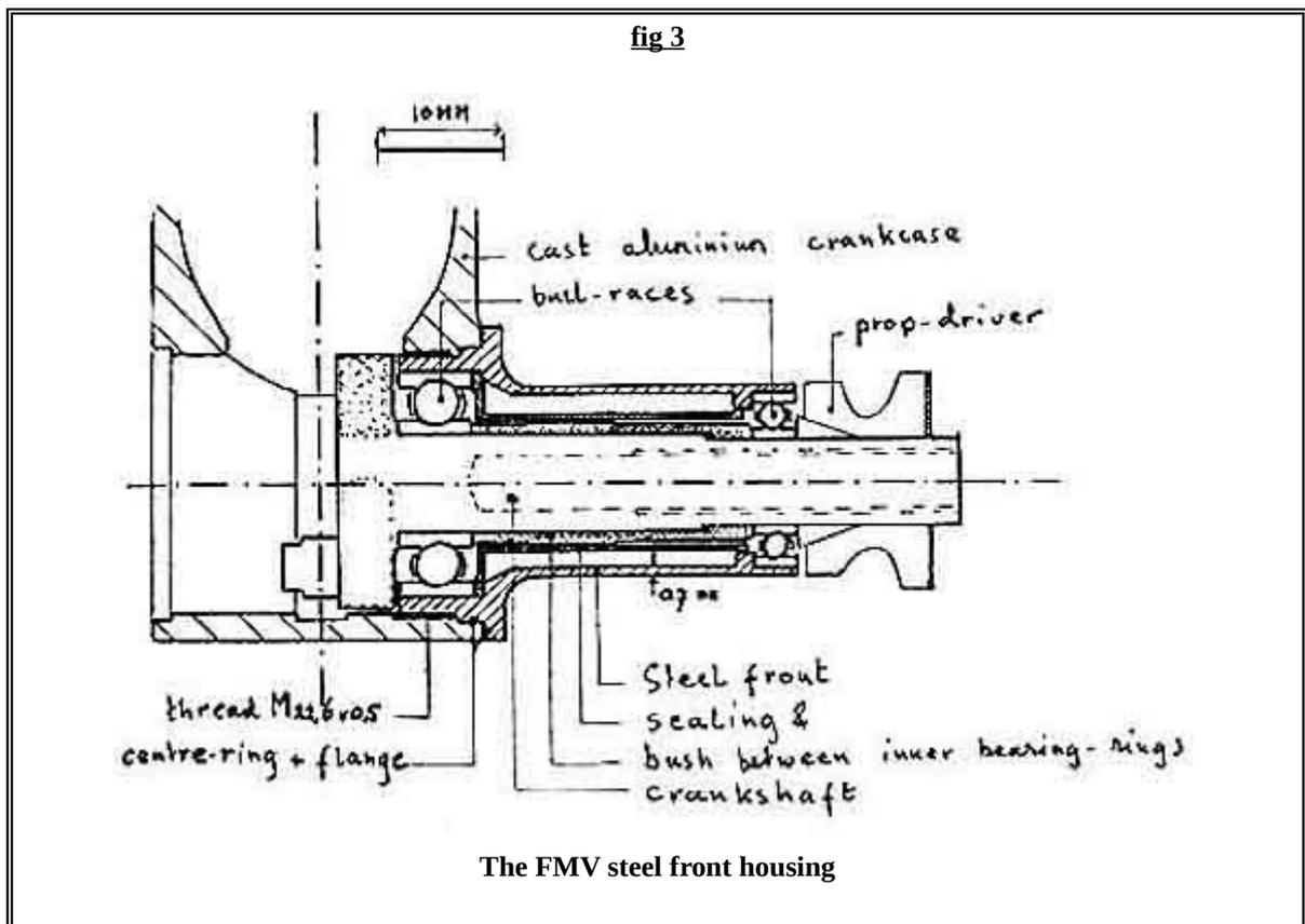
Getting the ballrace housings to size is an extremely accurate job, not helped by our deformable, normal clearance, bearings. With high clearance bearings more interference could be used and the relative accuracy of the house becomes less critical, but we still can't get these bearings in our sizes (8x19x6 and 7x14x3,5) without ordering large numbers.
