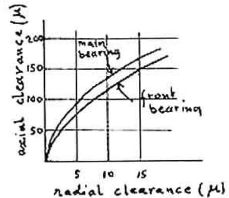
Curves of relationship between axial and radial clearance for Nelson bearings
