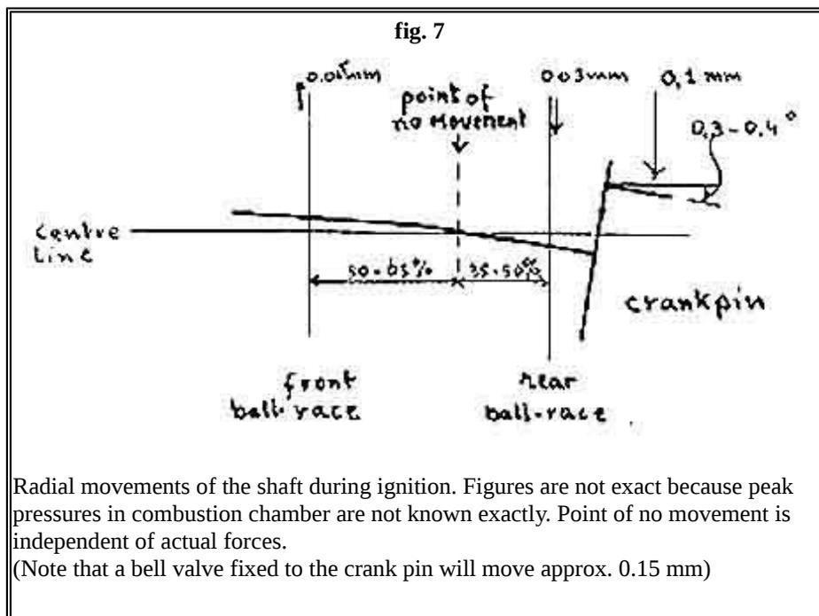
In any case it will be clear, that the best point of sealing the shaft is between the rear 1/3 and half the ball bearing center distance, where the movements are smallest. This is unlike most commercial RV-engines having the sealing right in front of the main bearing.
